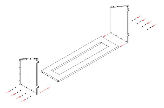
Place the base plate flat and fix the side plates to the base plate with the fasteners and washers provided. Do not tighten the fasteners completely. Hand fasten only as you might need to make a positioning and adjustments when the other plates are attached. Make sure the base plate front lip (without holes) is on the same side as the highest point of the side plates.
