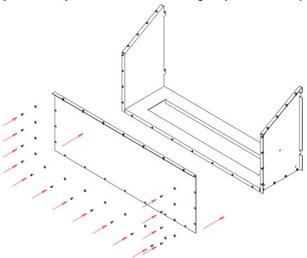
Next fasten the back plate to the base and side plates. Only hand tighten to allow for positioning and adjustments.
