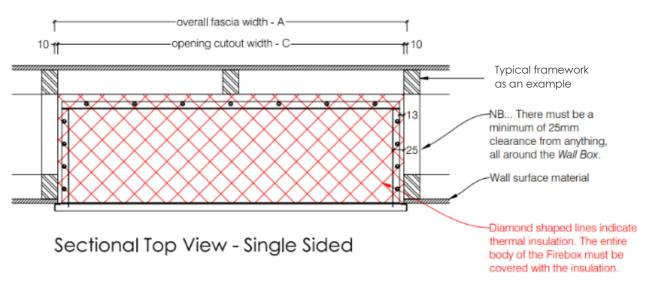
Note: The drawings above are an example of a typical installation using framework and covering the Firebox body with insulation. All installations must comply with the relevant building regulations and restrictions of the country where the installation is to take place.
